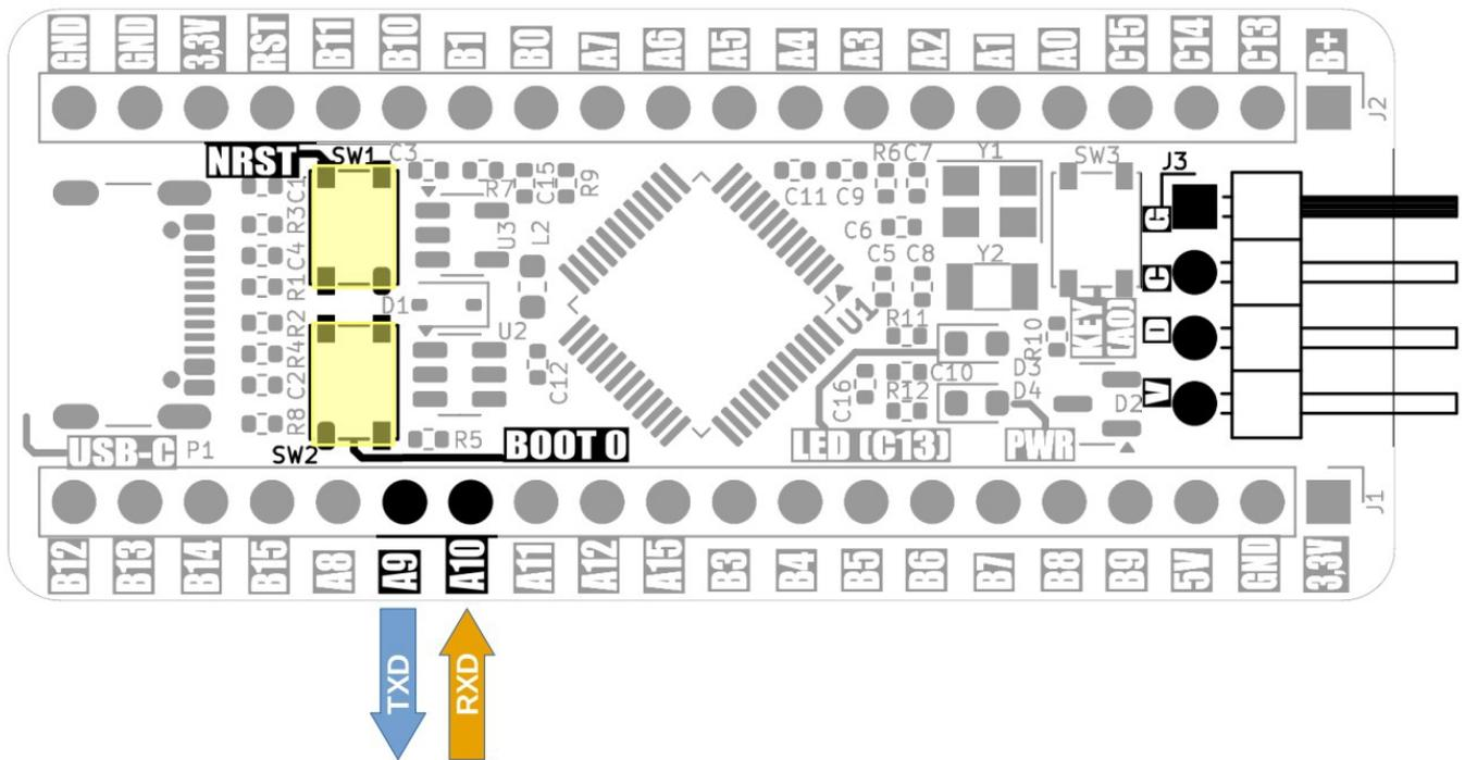
The **Kamod BluePill+** board also allows you to program the microcontroller via the USB interface using the Arduino IDE. This is possible because, along with the test program, an additional bootloader is placed in the program memory for communication and programming in the Arduino environment. Then you should:
